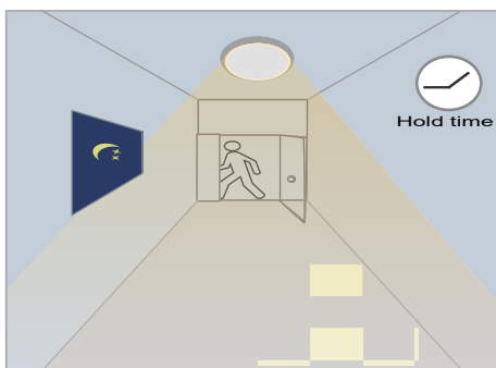
After the stand-by period, light OFF. After last detection, the light will be dimmed down to the stand-by dimming level (10%, 20%, 30% or 50%) after holdtime.
